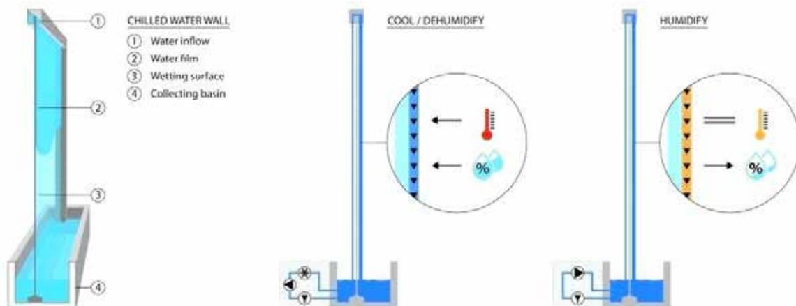
Fig.3. A representation of a watery wall details. Source: Fraunhofer Institute, 2018.
