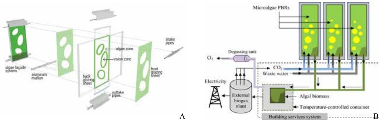
Fig. 5. A) demonstration of an algae façade's components. B) Operation mechanism of algae façade. Source: Elrayies, 2018.
