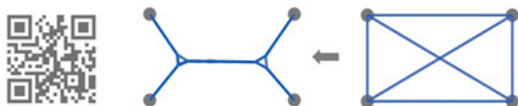
Fig. 7. All the possible direct paths, then the optimal path resulted from digital form-finding of the wet threads in the Grasshopper, and its simulation QR-code. Source: Authors.
