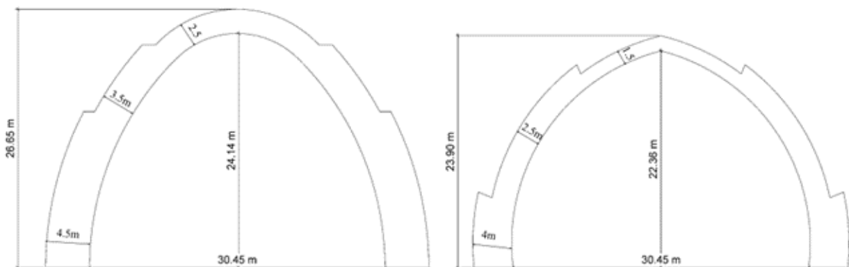
Fig. 6. Modeled dimensions of the opening, height, and thickness of the proposed pointed and parabolic arches of Alishah's Arch. Source: Safiri, 2025.
